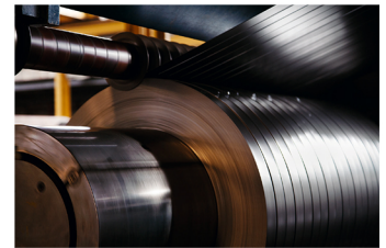
2014. Midland Steel, owned by the Allen family, is a beautiful brick factory, with 50+ foot ceilings. Servicing the eastern seaboard, it will 'level' and 'slitter' the rolled coils, which weigh 20,000-50,000 pounds. Steel was one of the first industries in in Hunts Point. As the city grew higher so did its demand for steel.
